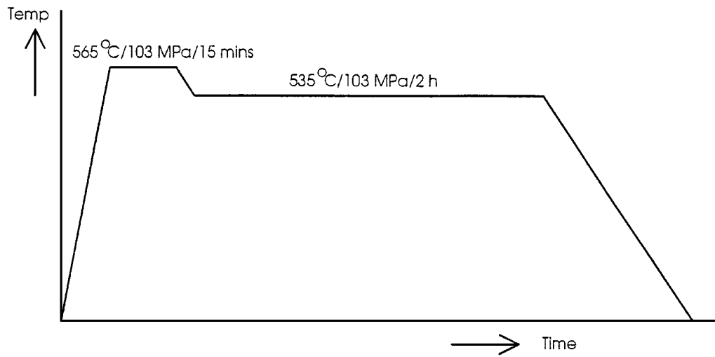
Figure 2 Temperature versus time profile for HIP cycle 3. The solidus is at 555°C and the liquidus for A357 at 615°C.
